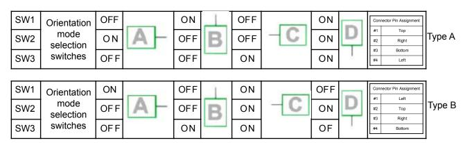
Connector Pin Assignment listed on individual touch panel drawings.
