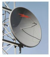
3.7 m | 12 ft Standard Parabolic Unshielded Antenna, dual-polarized, 10.500–10.700 GHz, CPR90G, gray antenna, with flash, standard pack—two-piece reflector
