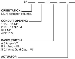
L1 Roller Lever L2 Rod Lever L3 One Way Roller Lever L4 Manual Lever P1 Straight Plunger, Std. W1 Coil Spring Wobble W2 Plastic Wobble, Std. W3 Plastic Wobble, Tall W4 Spring Wire, Std. W5 Spring Wire, Tall **SEALING PACKETS** (for use with the 1/2-14 npt conduit opening)
