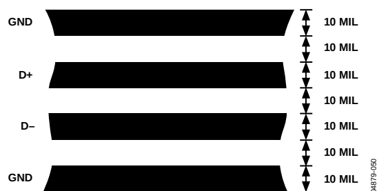
Figure 50. Arrangement of Signal Tracks
