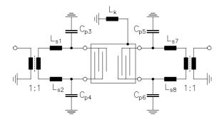
$$\begin{split} &L_{s1} = L_{s2} = 18 \text{ nH} \\ &C_{p3} = C_{p4} = 1.2 \text{ pF} \\ &C_{p5} = C_{p6} = 1.2 \text{ pF} \\ &L_{s7} = L_{s8} = 18 \text{ nH} \\ &L_{k} = 68 \text{ nH} \end{split}$$
