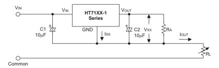
$$I_{OUT} = \frac{V_{XX}}{R_{\Delta}} + I_{SS}$$
