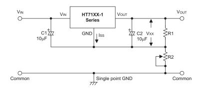
$$V_{OUT} = V_{XX} (1 + \frac{R2}{R1}) + I_{SS} R2$$
