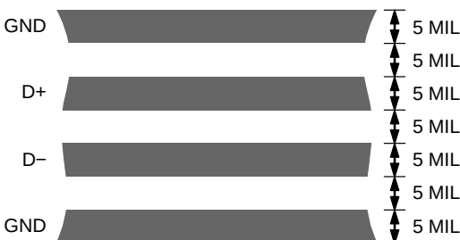
Figure 21. Typical Arrangement of Signal Tracks
