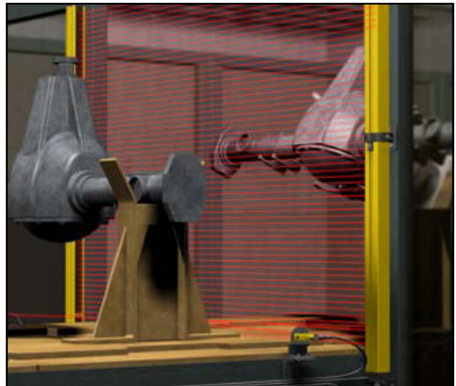
Figure 1-1. A typical EZ-SCREEN application: weld cell
