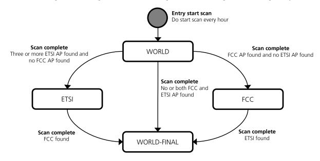
Figure 2: ODIN-W2 series IEEE 802.11d state transition diagram
