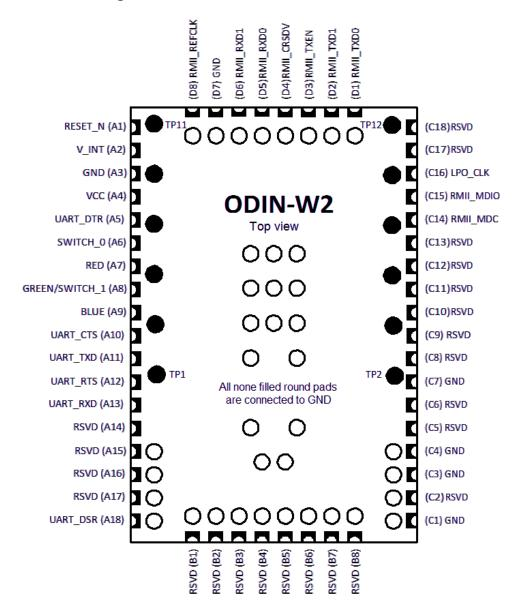
Figure 4: ODIN-W2 series pin assignment
