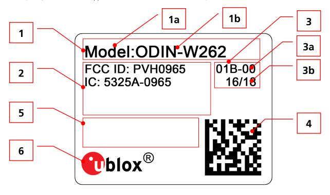
Figure 10: Location of product type number on the ODIN-W2 series module label
