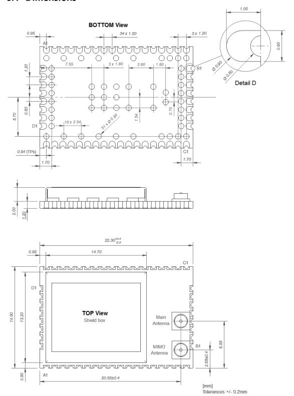
Figure 5: Physical dimensions of ODIN-W260
