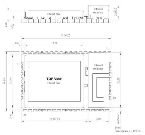
Figure 6: Physical dimensions of ODIN-W262
