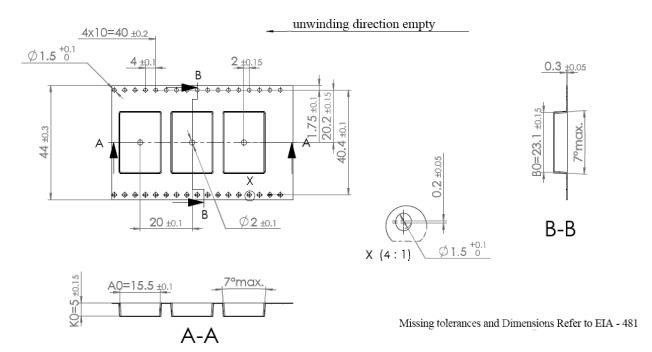
Figure 9: ODIN-W2 series tape dimensions
