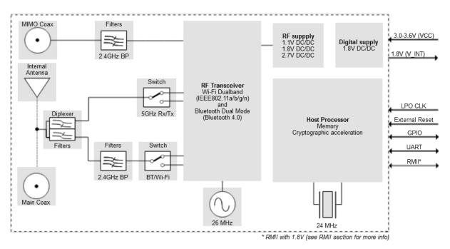
Figure 1: Block diagram of ODIN-W2 series
