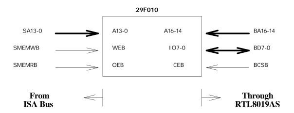
In this case, the BROM page mode is used. Before either to read or write BROM, the appropriate ROM page must be set in the BPAGE (page3, offset 02h) register first. The RTL8019AS will always reflect the content of BPAGE onto the BA14-21 bus. When RTL8019AS decodes a valid BROM read or write command, it asserts BCSB low. Note the flash memory write must be enabled through the RTL8019AS's FMWP register before the host's flash write command.
