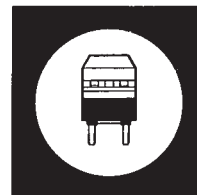
Stand-Off Lugs Minimize Solder-Creepage
