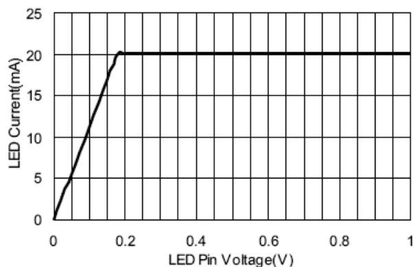
LED Current VS Input Voltage
