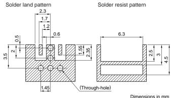
Dimensions in mm Tolerance:±0.13
