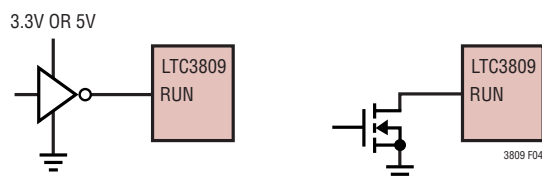
Figure 4. RUN Pin Interfacing
