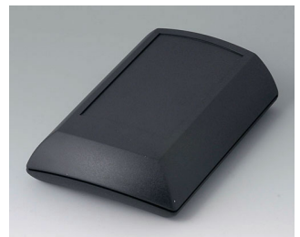
B7010209 ERGO-CASE M, flat ABS (UL 94 HB) black RAL 9005 5.91"x3.94"x1.57" IP 54 opt.
