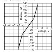
9. Off state leakage current Measured portion: between terminals 4 and 6; Ambient temperature: 25°C 77°F
