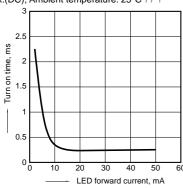
11. LED forward current vs. turn off time characteristics
