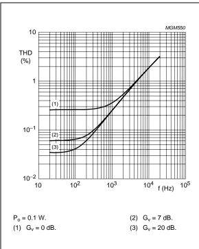
Fig.8 Total harmonic distortion as a function of frequency at different gains.
