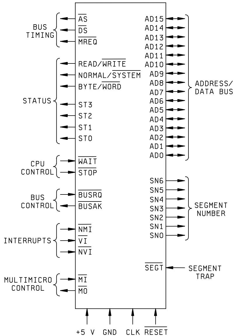
FIGURE 3. Logic functions.
