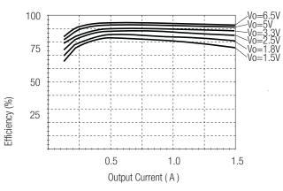
Efficiency Vs Load (Vin=Max)
