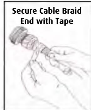
g) Open up the constant force spring and wrap it around the cable braid section that is positioned over the constant force spring slot area of the adaptor. This is most easily accomplished by lifting up the end of the spring and trapping the braid covered adaptor between the spring coil and raised end. The spring will now stay in place and can be installed by simply rolling the spring coil around the braid covered adaptor.
