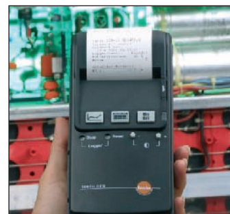
On site documentation of limits exceeded caused by fluctuations in ambient conditions e.g. during storage
