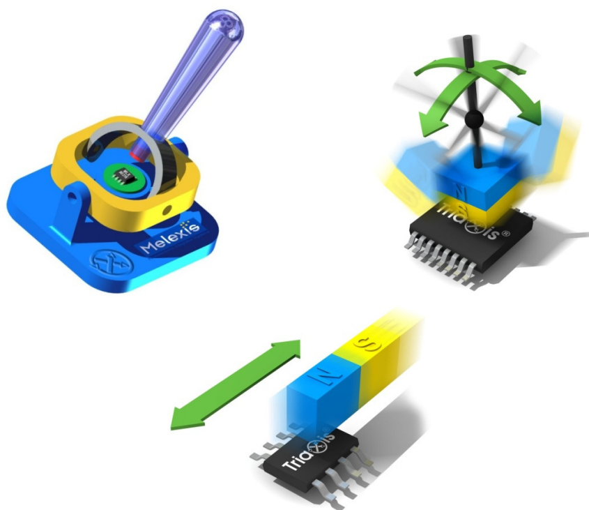
Figure 3 - Typical application of MLX90333
