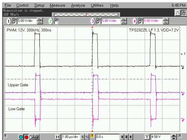
Figure 22. 12-V PWM Pulse at V_{DD} = 7.2 V
