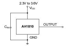
Note: 4. C<sub>IN</sub> is for power stabilization and to strengthen the noise immunity, the recommended capacitance is 10nF to 100nF.
