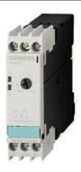
TIME RELAY, SOLID-STATE, ON-DELAY, 1 CHANGEOVER CONTACT, 1 TIME RA 0.5S TO 10S, AC 24, 200 TO 240V AND DC 24V, WITH LED, SCREW TERMINAL
