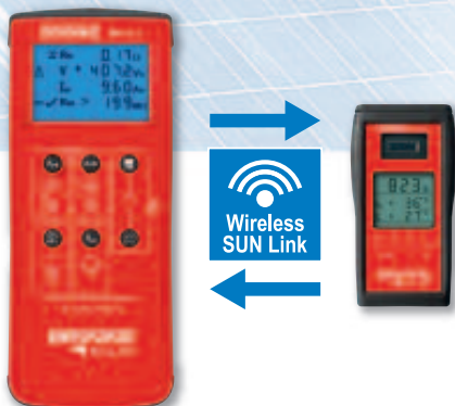
Wireless transmission of measuring data (alternatively import of measuring data by means of date/time stamp)
