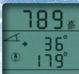
Insolation, angle of inclination and compass bearing
