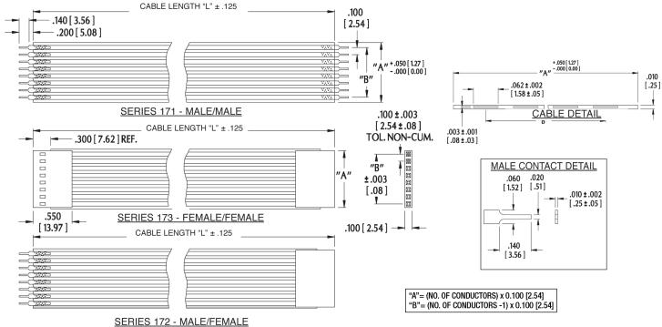
ALL DIMENSIONS: INCHES [MILLIMETERS] ALL TOLERANCES: ±0.005 [0.13] UNLESS OTHERWISE SPECIFIED FOR CABLE LENGTHS UNDER 2.000 [50.80], CONSULT FACTORY FOR 90° PIN STAKED FLEX JUMPERS, SEE DATA SHEET 11019 FOR Rohs applications, use HT cable CONSULT FACTORY FOR OTHER SIZES AND CONFIGURATIONS
