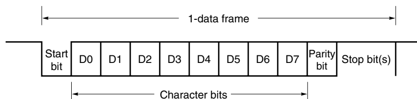
Figure 16-7. Format of Asynchronous Serial Interface Transmit/Receive Data
