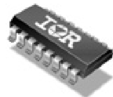
16-Lead SOIC (Narrow Body)
