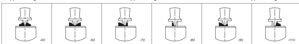
Note : -5V and -12V are not true locking levers : no pulling is required before actuation.
