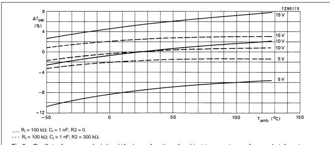
Fig.9 Oscillator frequency deviation ( $\Delta f_{osc}$ ) as a function of ambient temperature; referenced at:  $f_{osc}$  at  $T_{amb} = 25$  °C and  $V_{DD} = 10$  V.
