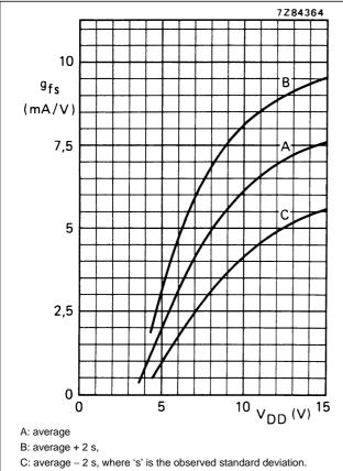
Fig.7 Typical forward transconductance  $g_{fs}$  as a function of the supply voltage at  $T_{amb} = 25 \, ^{\circ}C$ .
