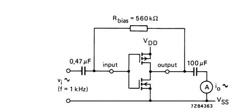
Fig.6 Test set-up for measuring forward transconductance  $g_{fs} = di_o/dv_i$  at  $v_o$  is constant (see also graph Fig.7); MR = LOW.
