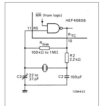
Fig.5 External component connection for crystal oscillator.
