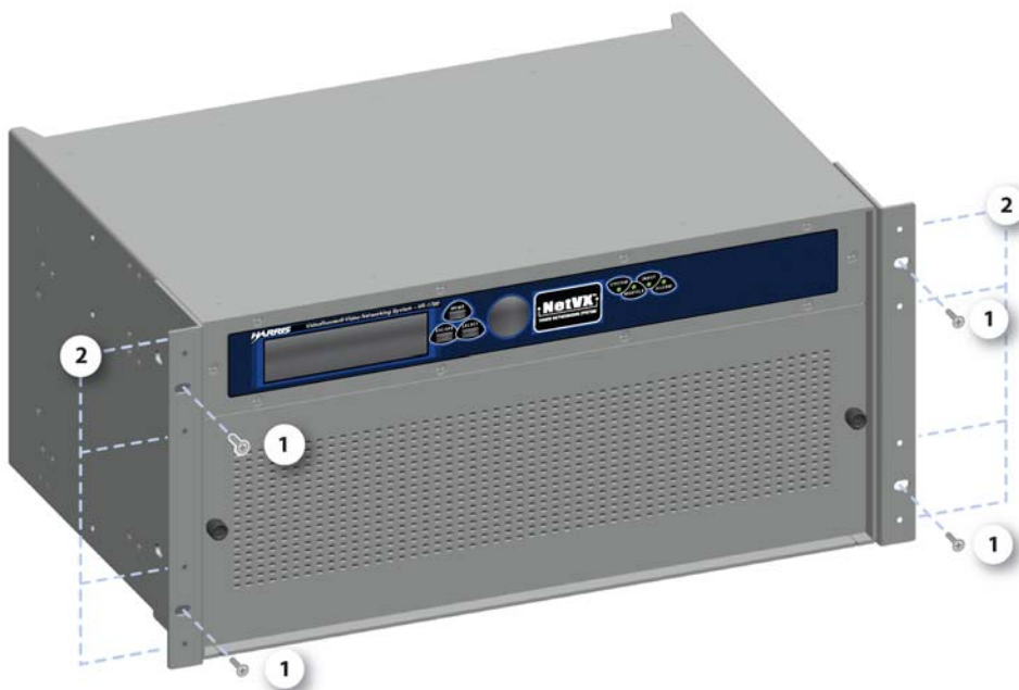
Figure 6-1 SYS-1700 Rack Mount Screw Locations
