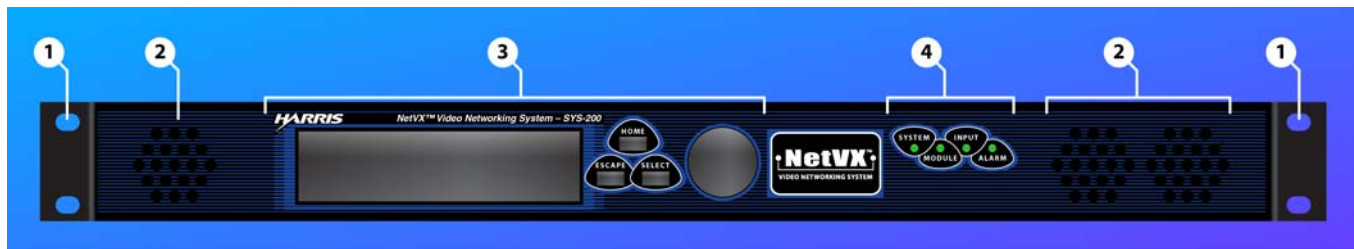
Figure 3-1 SYS-200 Chassis – Front View
