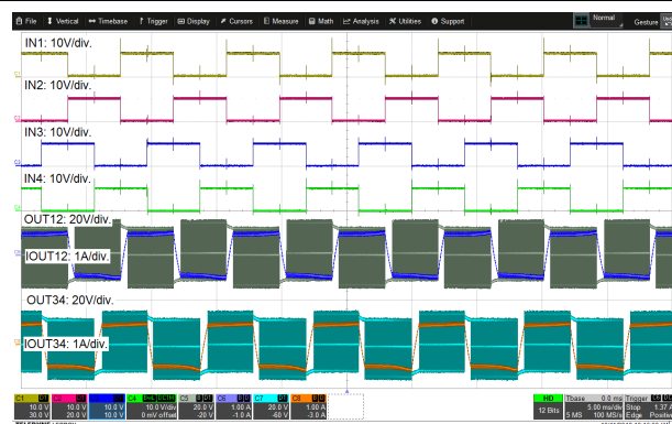
Figure 8-7. Stepper Motor Full-Step Operation
