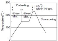
[Recommended condition for Pb-free soldering]
