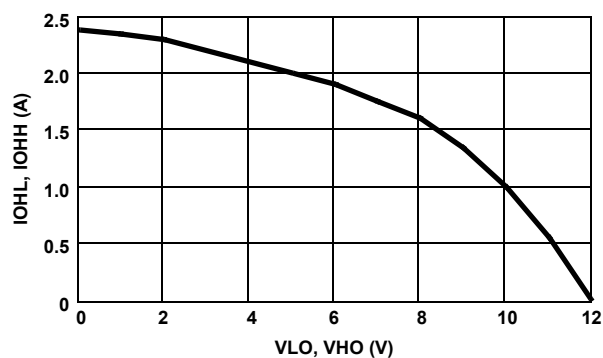
FIGURE 17. PEAK PULL-UP CURRENT vs OUTPUT VOLTAGE
