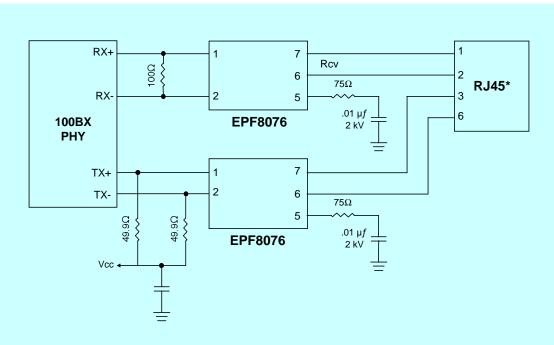
Notes: \* Pin-outs shown are for DCE configurations: e.g. Hubs, Repeaters
