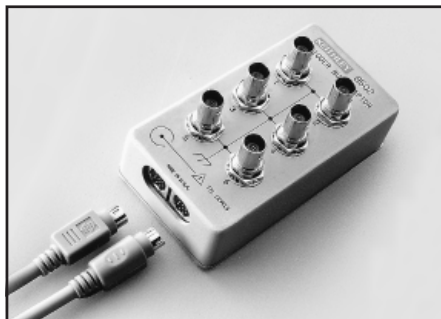
Model 8502: Trigger Link adapter box has two female 8-pin micro DIN connectors to 6 female BNC connectors. Includes an 8501-1 cable.
