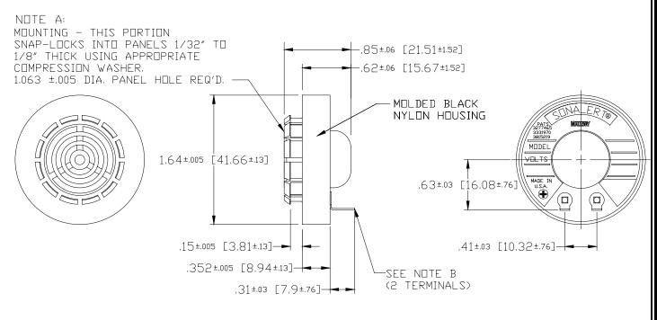
NOTE B: TERMINALS - .016 BRASS, HOT TIN FINISH WITH .076 WIRE HOLE, TERMINAL WILL ACCEPT STANDARD 1/8" QUICK CONNECT
