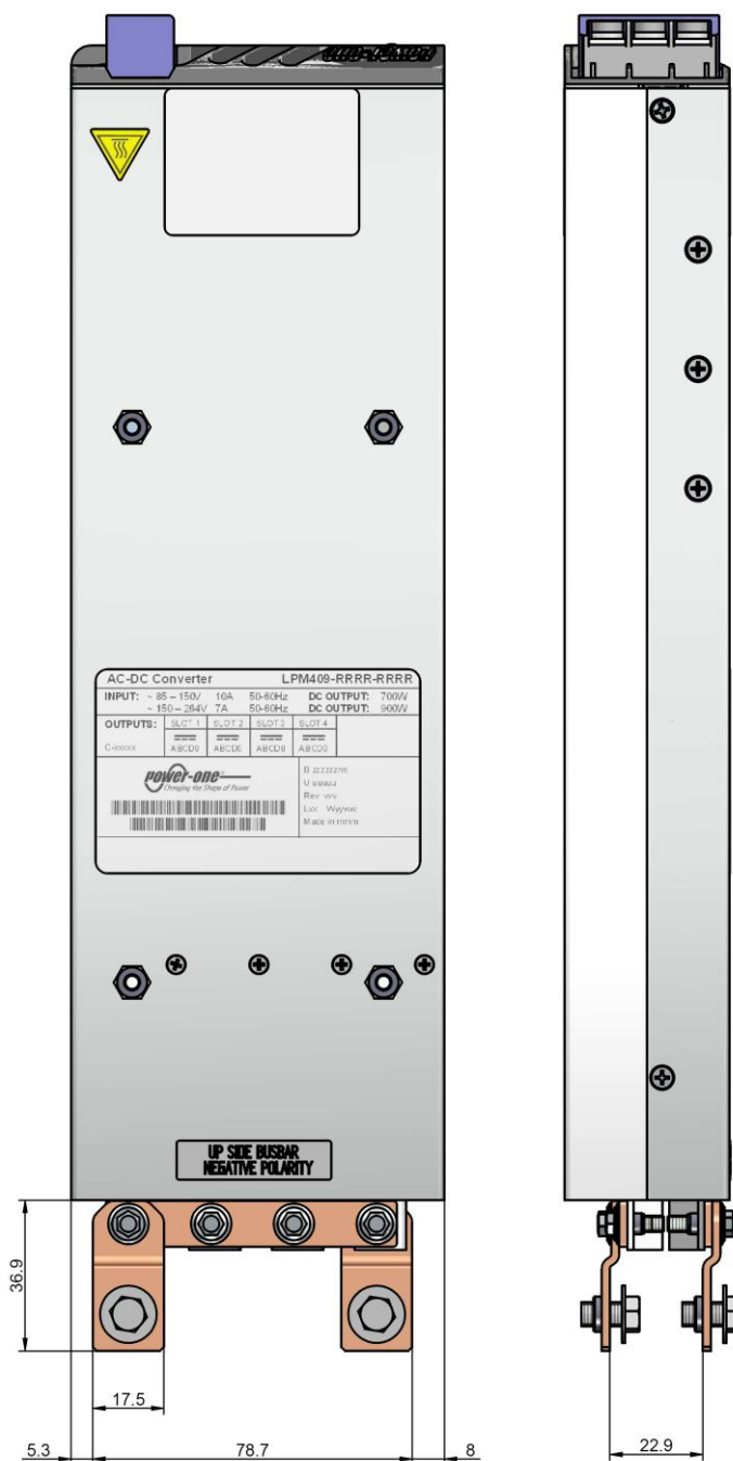
Figure 13. LPM409-AAAA-DXXX parallel configuration
