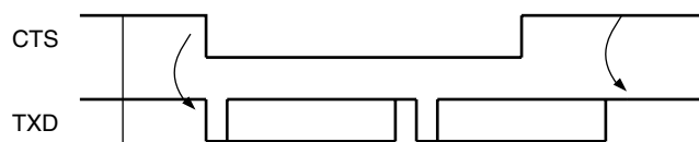
Figure 30-21. Transmitter Behavior when Operating with Hardware Handshaking
