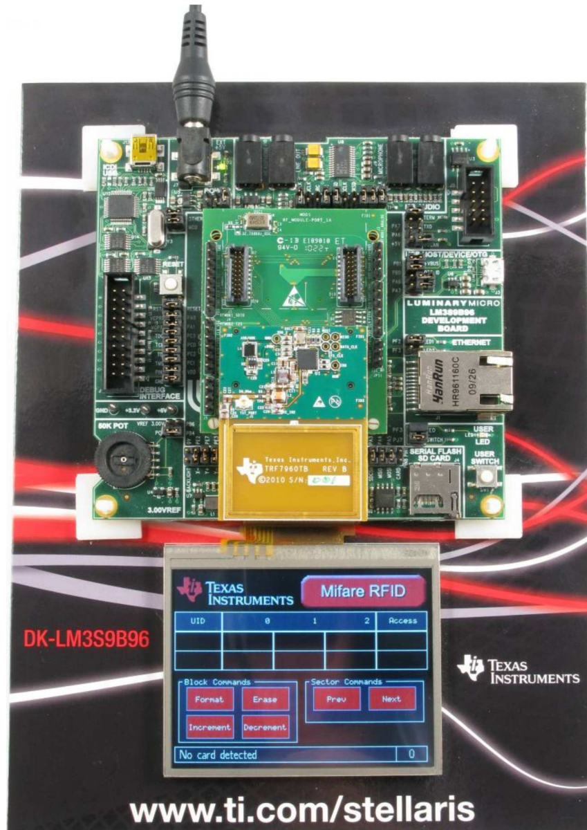
Figure 6. DK-LM3S9B96-EM2-TRF7960R Development Platform
