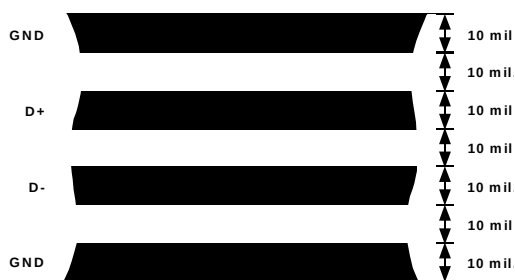
Figure 13. Arrangement of Signal Tracks
