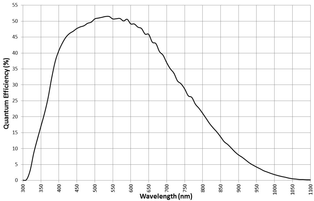
Figure 9. Monochrome QE with Microlens and MAR Glass
