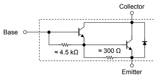
Electrical Characteristics ( $T_c = 25^\circ\text{C}$ )
