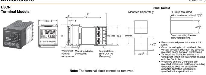
Note: The terminal block cannot be removed.
