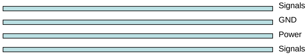
Figure 17: Typical 4-layer PCB construction
