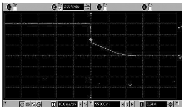
Fall Time (PWM mode): Vin = 4V; Vout = 6V; Iout = 1A
