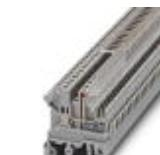
Feed-through terminal block, Nominal current: 12 A, Nominal voltage: 250 V, Cross section: 0.2 mm<sup>2</sup> - 4 mm<sup>2</sup>, AWG: 24 - 12, Mounting type: NS 32, NS 35/15, NS 35/7,5, Number of positions: 1, Pitch: 5.08 mm, Width: 5.1, Color: gray
