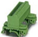
Plug component, Nominal current: 12 A, Rated voltage (III/2): 320 V, Number of positions: 21, Pitch: 5.08 mm, Connection method: Screw connection, Color: green, Contact surface: Tin, Assembly: DIN rail
