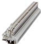
Feed-through terminal block, Nominal current: 12 A, Nominal voltage: 250 V, Cross section: 0.2 mm<sup>2</sup> - 4 mm<sup>2</sup>, AWG: 24 - 12, Mounting type: NS 35/7,5, NS 35/15, NS 32, Number of positions: 1, Pitch: 5.08 mm, Width: 5.08, Color: gray
