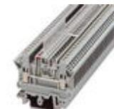
Feed-through terminal block, Connection method: Special and hybrid connection, Number of positions: 1, Cross section: 0.2 mm<sup>2</sup> - 4 mm<sup>2</sup>, AWG: 24 - 12, Width: 5.08 mm, Color: gray, Mounting type: NS 32, NS 35/15, NS 35/7,5
