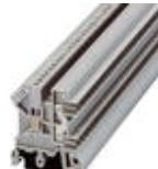
Feed-through terminal block, Connection method: Special and hybrid connection, Number of positions: 1, Cross section: 0.2 mm<sup>2</sup> - 4 mm<sup>2</sup>, AWG: 24 - 12, Width: 5.08 mm, Color: gray, Mounting type: NS 32, NS 35/15, NS 35/7,5
