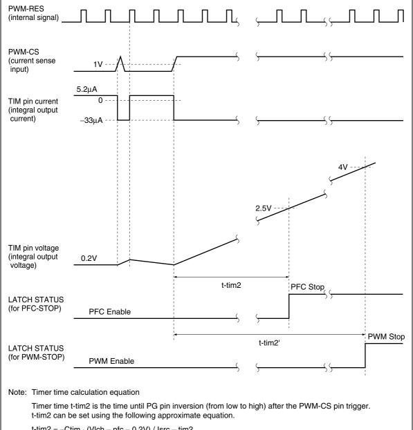
$$\begin{array}{l} \text{t-tim2} = -\text{Ctim} \cdot (\text{Vlch} - \text{pfc} - 0.2\text{V}) \, / \, \text{Isrc} - \text{tim2} \\ = -\text{Ctim} \cdot (2.5\text{V} - 0.2\text{V}) \, / \, (-33\mu\text{A}) \cdot \cdot \cdot \cdot \cdot \, \text{Typical calculation} \end{array}$$
