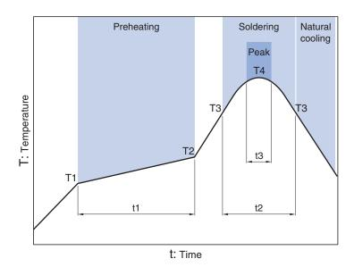
Soldering Preheating Peak Temp. Time Time Temp. Time Temp. T2 **T3** T4 t3 150°C 180°C 60 to 120s 220°C 40s 260°C 5s
